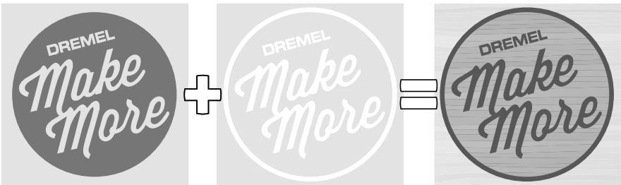
dark engrave (image file) + text outline (vector file) = text and circle cut out
